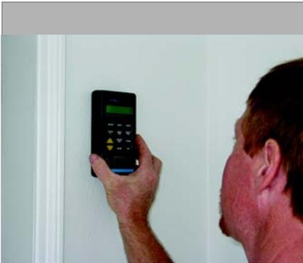
Many inspectors perfect their inspection techniques by choice of tools. This technician has wisely chosen a moisture meter to locate moisture behind walls.
